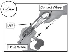
Figure 6. Attaching the sanding belt.
